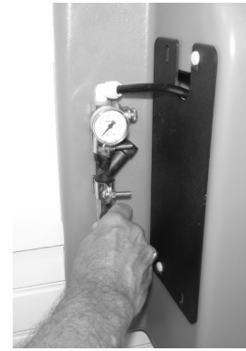
9. Turn on the water supply. Adjust the pressure regulator as needed.
